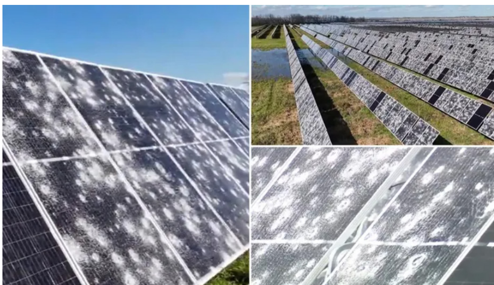
Figure 5. Damage to Solar Panels After Hailstorm with Abnormally Large Hailstones (April 15, 2024, Texas, USA)
